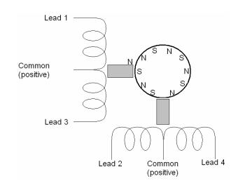
The leads that provide current to each coil are always color coded, but the codes are different for different manufacturers and even for different models made by the same manufacturer. Color codes for some of the motors we use are shown below, numbered to correspond with our programs for the Motor Controller.
