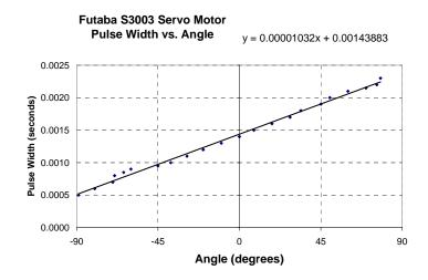
values can be very different for different brands and models of motors, sometimes even reversing positive and negative movements. The calibration can also be different even among servo motors that are the same brand and model. They really do need to be calibrated individually to achieve the maximum effectiveness.
